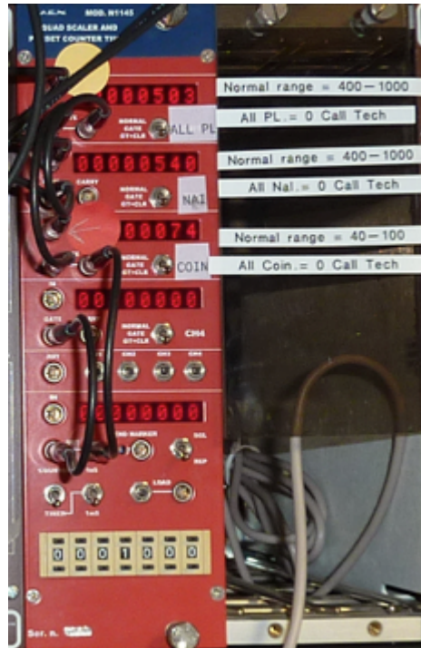
Figure 43. CAEN signal counter depicting summed plastic, NaI, and coincidence values.
