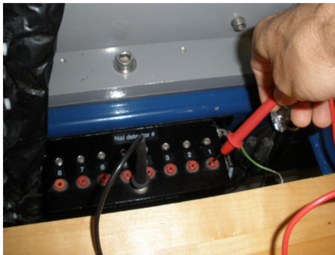
Figure 9. Insert the multimeter probes into the bias detector box to measure the voltage. Black to white. Red to red
