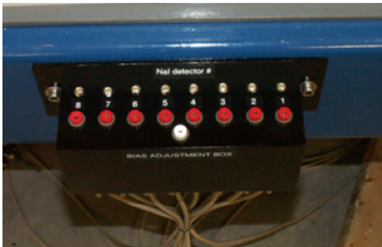
Figure 8. NaI bias adjustment box
