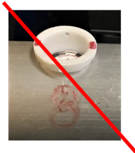
Figure 7. Don't place the plastic holder in hole 8 or 1, it can damage the NGRL.
