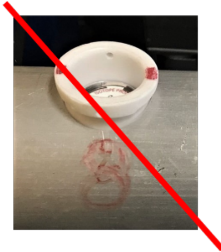
Figure 30. Don't place the plastic holder in hole 8 or 1, it can damage the NGRL.
