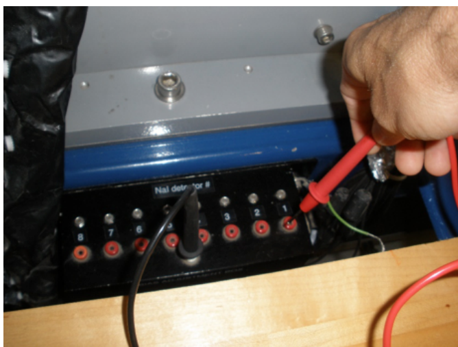
Figure 27. Insert the multimeter probes into the bias detector box to measure the voltage. Black to white. Red to red
