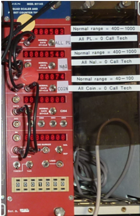
Figure 7. CAEN signal counter depicting summed plastic, NaI(Tl), and coincidence values
