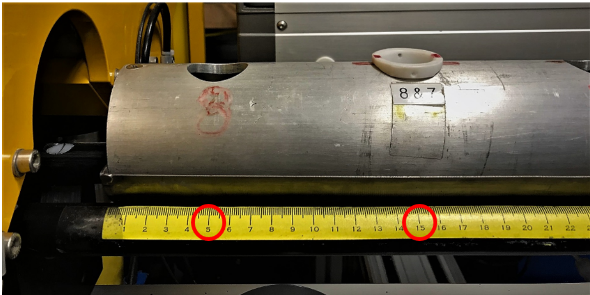
Figure 29. Calibration offsets for non-collimated sources: For placing the sources between detectors use a 5 cm offset. For placing the sources on top of detectors use a 15 cm offset.
