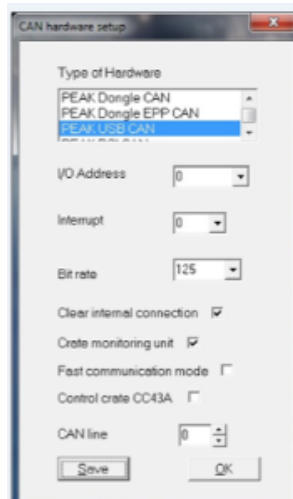
Figure 13a. iSEG Hard ware Setup and Main screen
