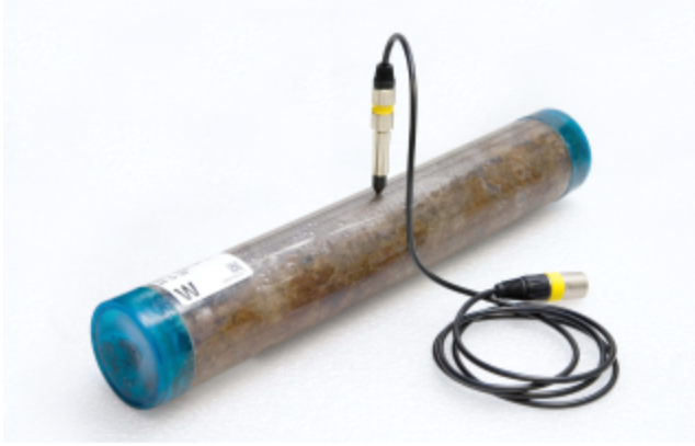
Figure 2. Thermal conductivity measurement on a soft-sediment section using full-space probe.
