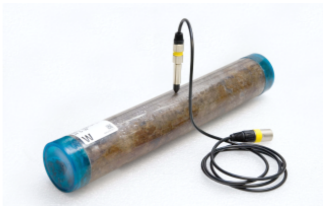
Figure 1. Thermal conductivity measurement on a soft-sediment section using full-space probe.
