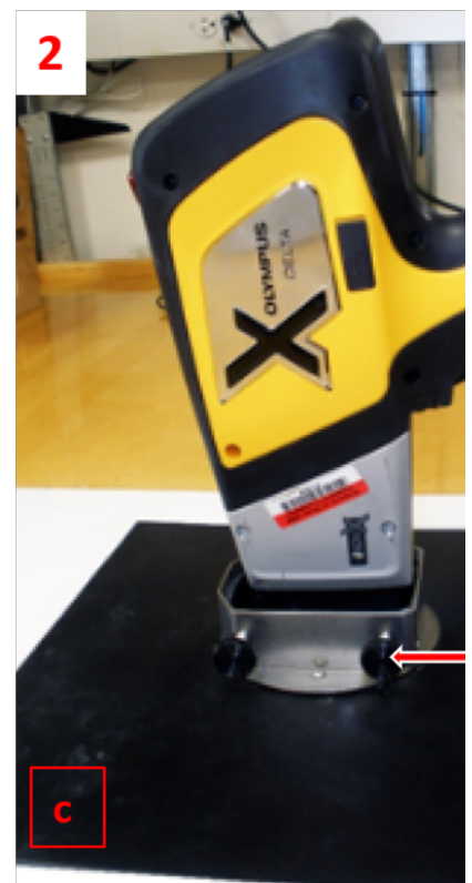
Figure 11. Sample Chamber (a) snaps into the gun of the nose for measuring discrete samples (1). Leaded Shielding(c) for Section Half measurements (2). The nose of the gun goes into the opening and is tightened with the side screws(d).
