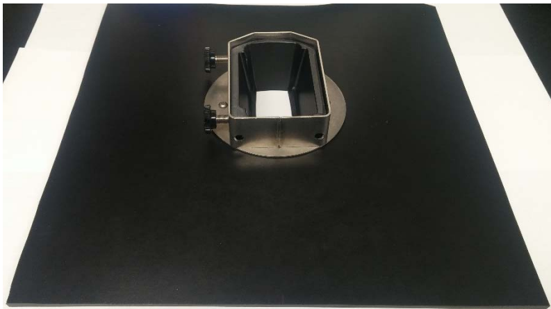
Figure 10. Leaded Shielding for Section Half measurements. The Nose of the gun goes into the opening and is tightened with the side screws.
