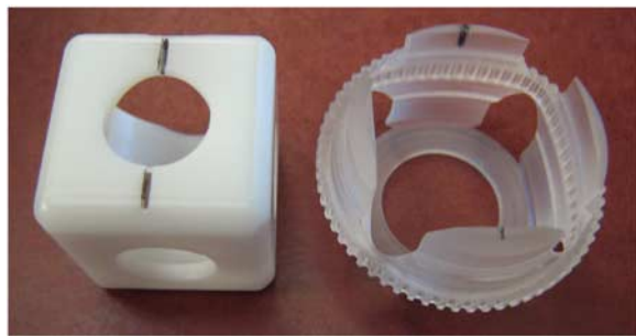
Figure A4. Cubic specimen holder and cog used for positioning standard 2.54 cm diameter cores.
