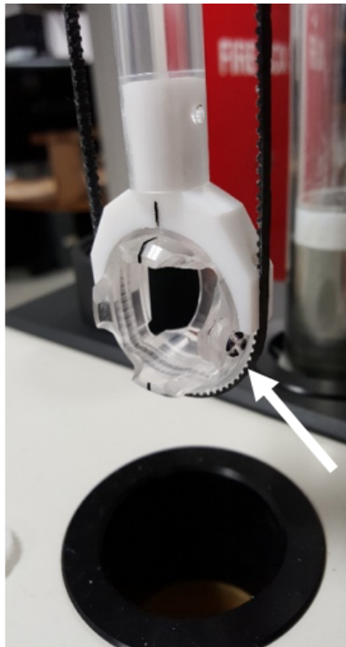
Figure 12. Empty Kappabridge Holder prepared for holder measurement. Note that the screw (indicated by white arrow) must be flush with the holder before starting the measurement.
