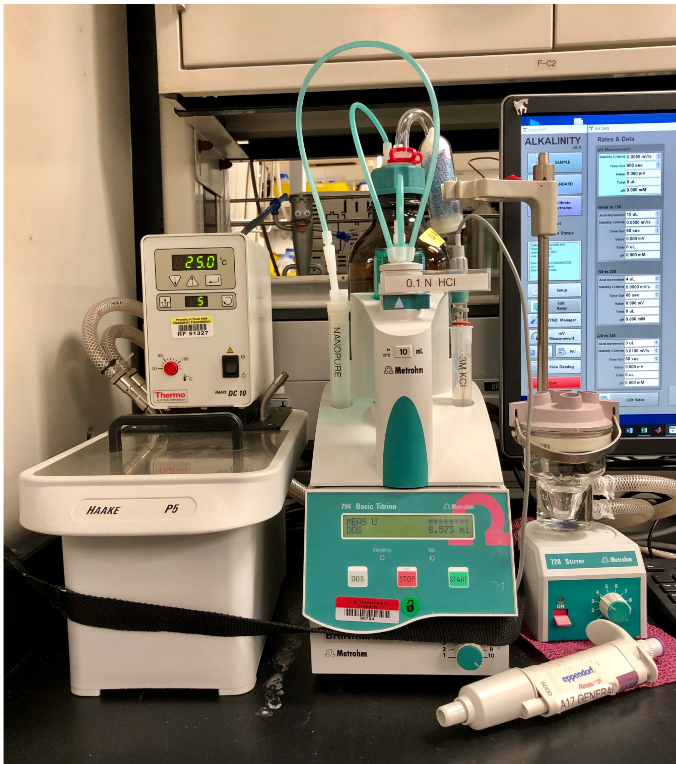
Figure 1. Metrohm Autotitrator (Note: dispenses 0.1 M HCl).
