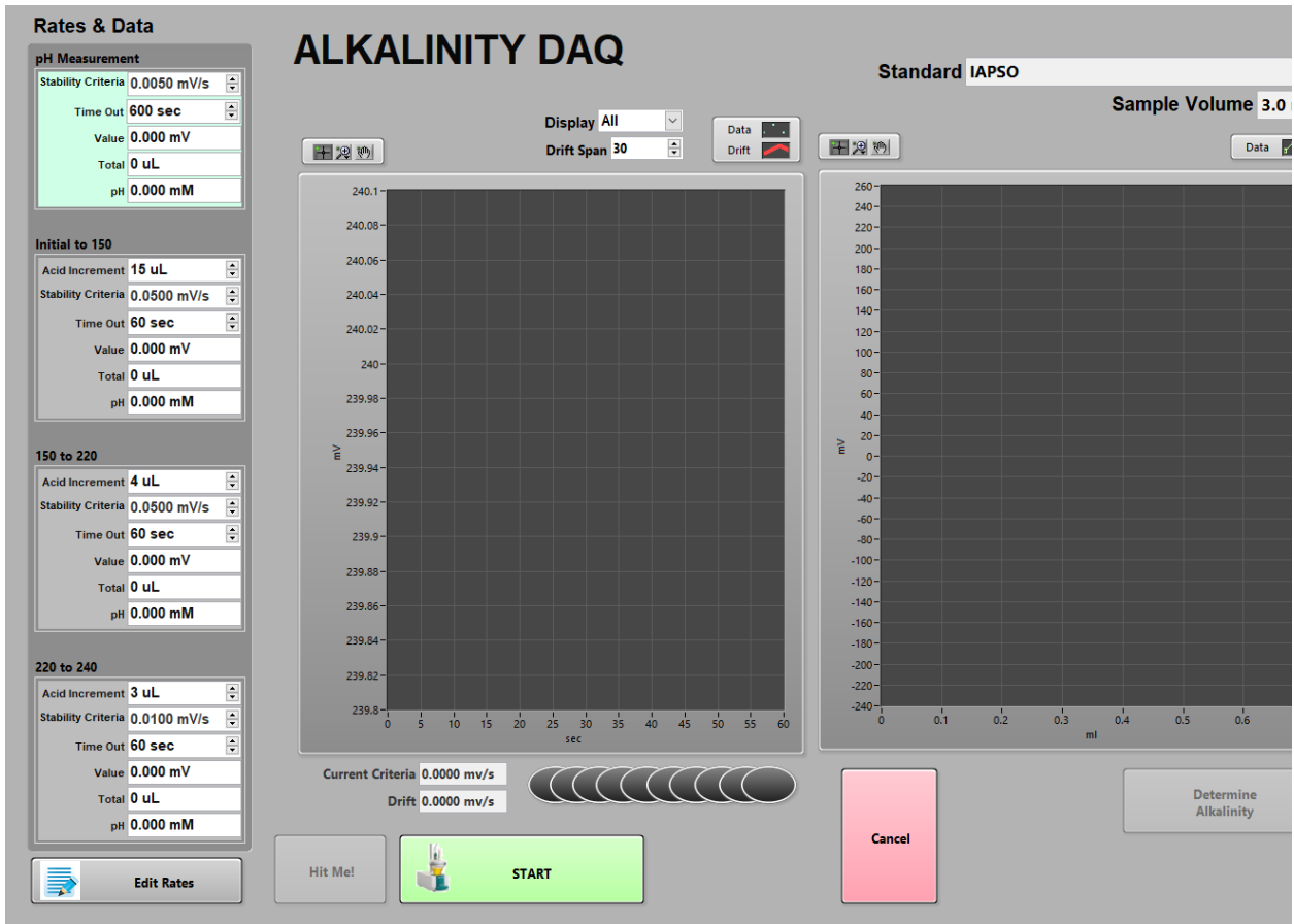
Figure 6. Measuring a standard for standard ratio correction.
