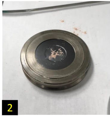
2. Putting sample powder in the middle of a zero background Si disk
