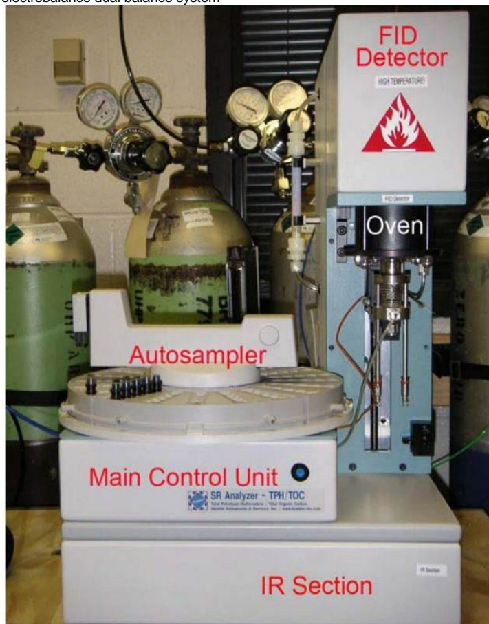
Figure 1. Main Components of the SRA System.
