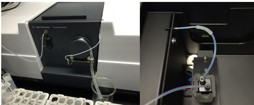
Figure 1 : Sample inlet tube and flow cell
