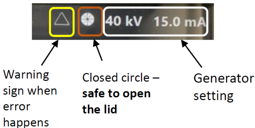
Figure 1. Aerial touchscreen safety information. The closed circle icon on the screen indicates when the shutter is closed and it is safe to open the lid.
