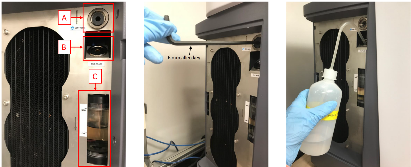
Figure 35. Cooling fluid reservoir. A. Vent plug, B. Fill plug, C. Coolant reservoir.
