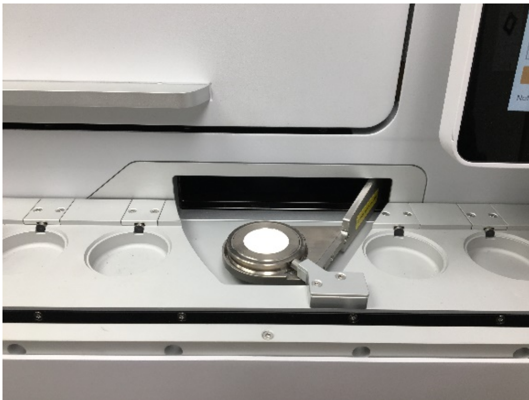
Figure 26. Manual Mode, one sample at a time placed directly on the sample changer arm.
