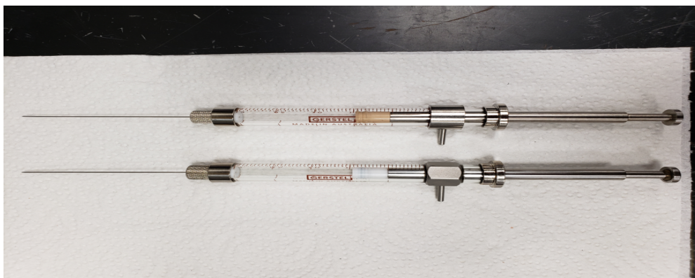
Figure 6: Different syringes used by the Gerstel Autosampler. The rubber plunger of the syringe shown on top causes significant sample carryover, likely due to tracer penetrating pore spaces within the rubber. It is best to use the syringe with the teflon-tipped plunger shown on bottom.
