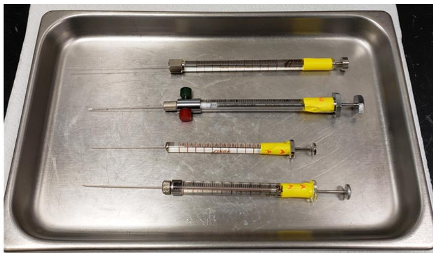
Figure 5: Different syringe types for preparing PFT standards and for injecting samples. Listed from top to bottom: 1  $\mu$ L glass analytical syringe from Scientific Glass Engineering (SGE), 0.5 mL Teflon-fitted Pressure-Lok glass syringe from Precision Sampling Corp, 10  $\mu$ L glass analytical syringe from SGE, 0.10 mL (100  $\mu$ L) Microliter #710 glass syringe from Hamilton Co.
