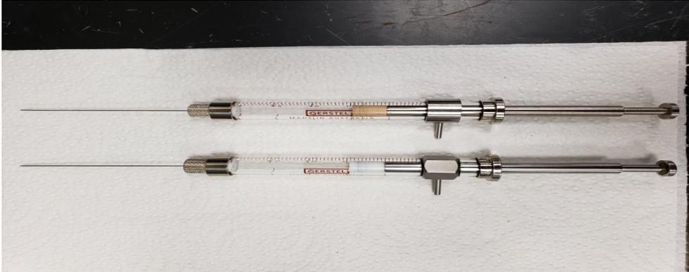
**Figure 6: Different syringes used by the Gerstel Autosampler. The rubber plunger of the syringe shown on top causes significant sample carryover, likely due to tracer penetrating pore spaces within the rubber. It is best to use the syringe with the teflon-tipped plunger shown on bottom.**
