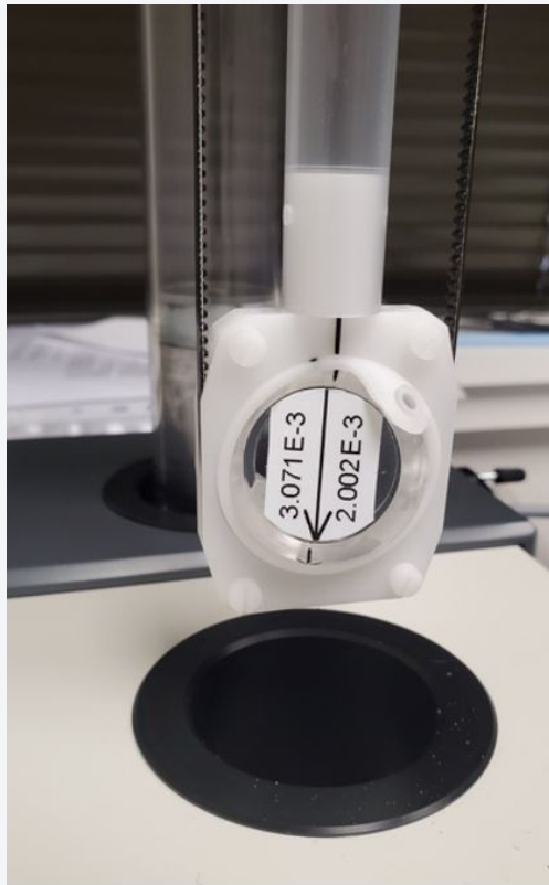
Figure 15: Calibration standard in the 3D holder
