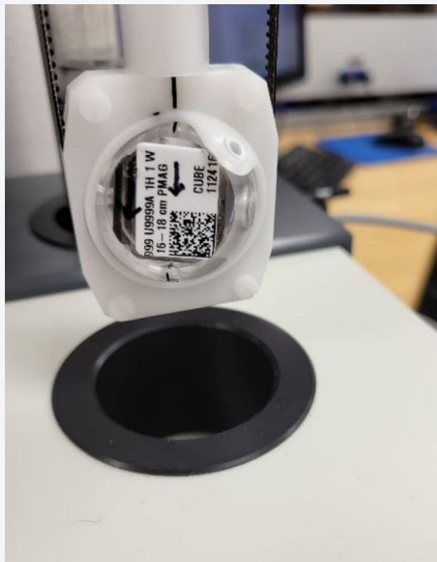
Figure 26: Sample in 3D Holder using the Cylinder setting
