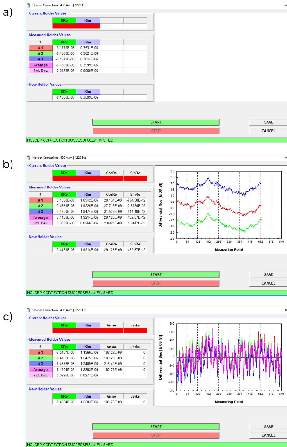
Figure 14: Typical examples of the Holder Correction windows for a) Manual measuring modes (including Manual Anisotropy Mode), b) 1-Axis Rotator, c) 3D Rotator.
