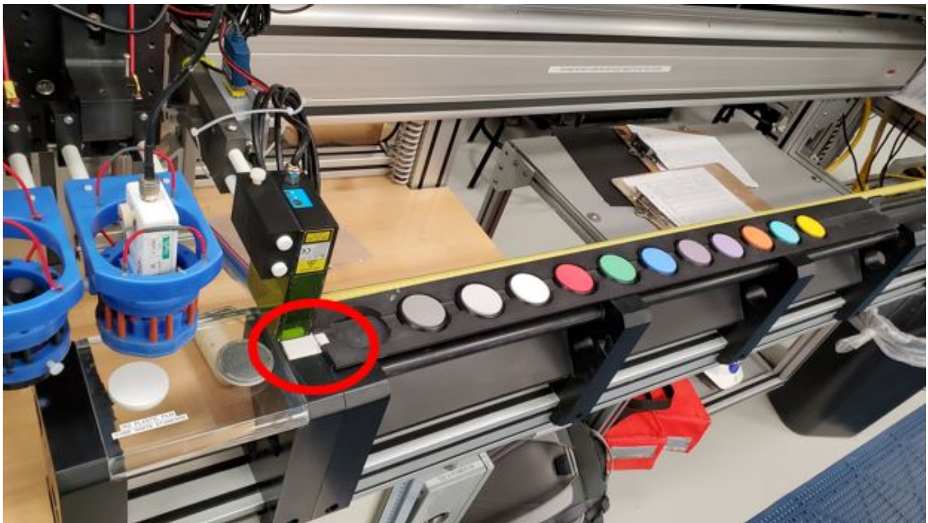
Figure 30 - Color Reflectance Control Set on SHMSL track. The white square on the end of the standard holder should be against the white benchmark (red circle).
