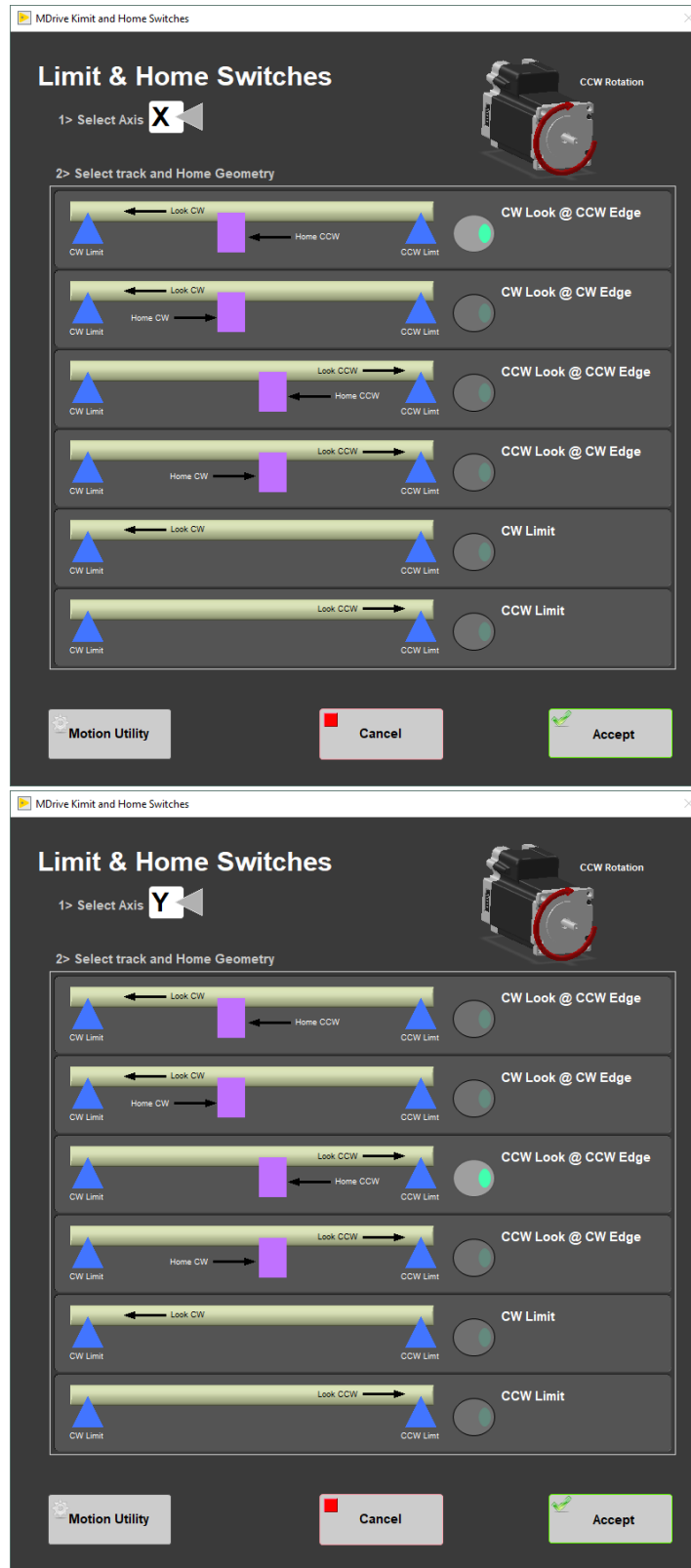
Figure 44. X-Axis (left) and Y-Axis (right) Limit and Home Switch Configuration
