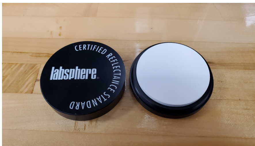
Figure 40. WHITE Spectralon® Calibration Standard
