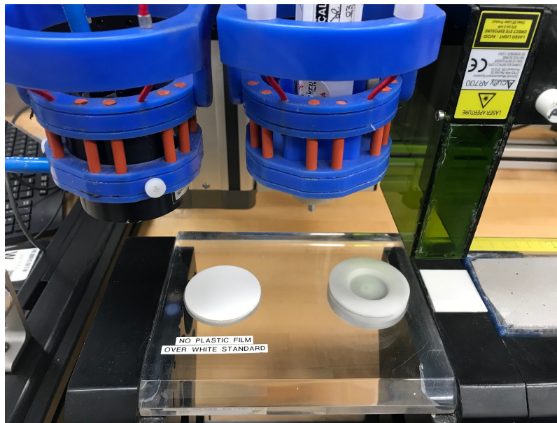
Figure 6. White color reflectance standard calibration (left) and MS standard (right).
