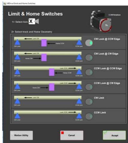
Figure 18. Limit and Home Switch Configuration
