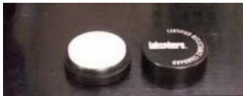
Figure 35. WHITE Spectralon® Calibration Standard
