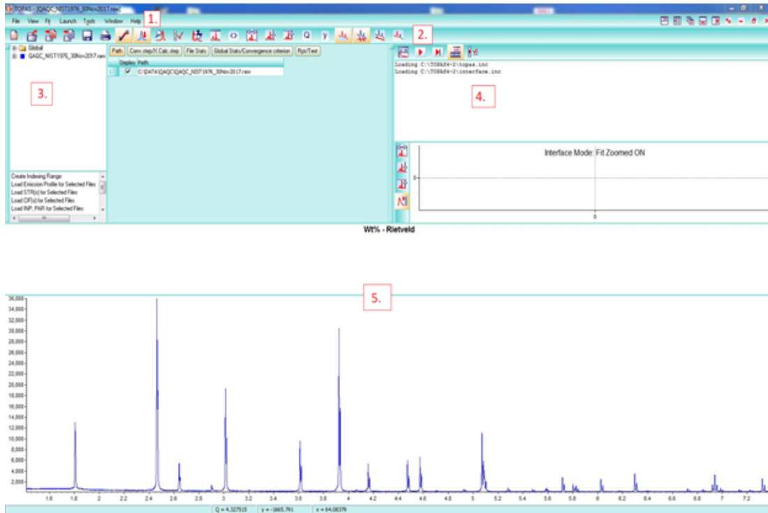
Figure 2. Main window of TOPAS with Scan loaded. 1. Menu Bar 2. Toolbar 3. Parameter Window 4. Fit Window 5. Main Work Area
