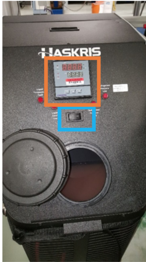
Figure 8: Haskris Water Chiller with water tank open. Water surface should be clean. Do not pump dirty water through the Haskris.
