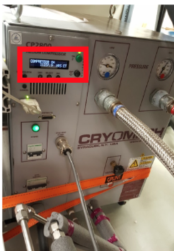
Figure 7: Cryomech Compressor for SRM. Red box indicates display which will indicate a low flow error if cooling water is not circulating to the compressor.
