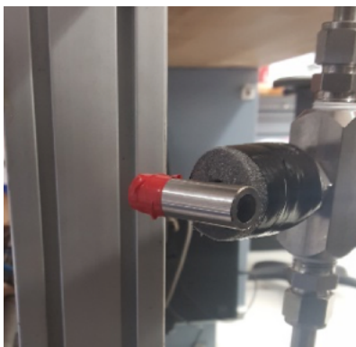
Figure 6: Metering valve for the ship's chill water. The red tape is used as a reference when adjusting the valve. All adjustments should be small and incremental.
