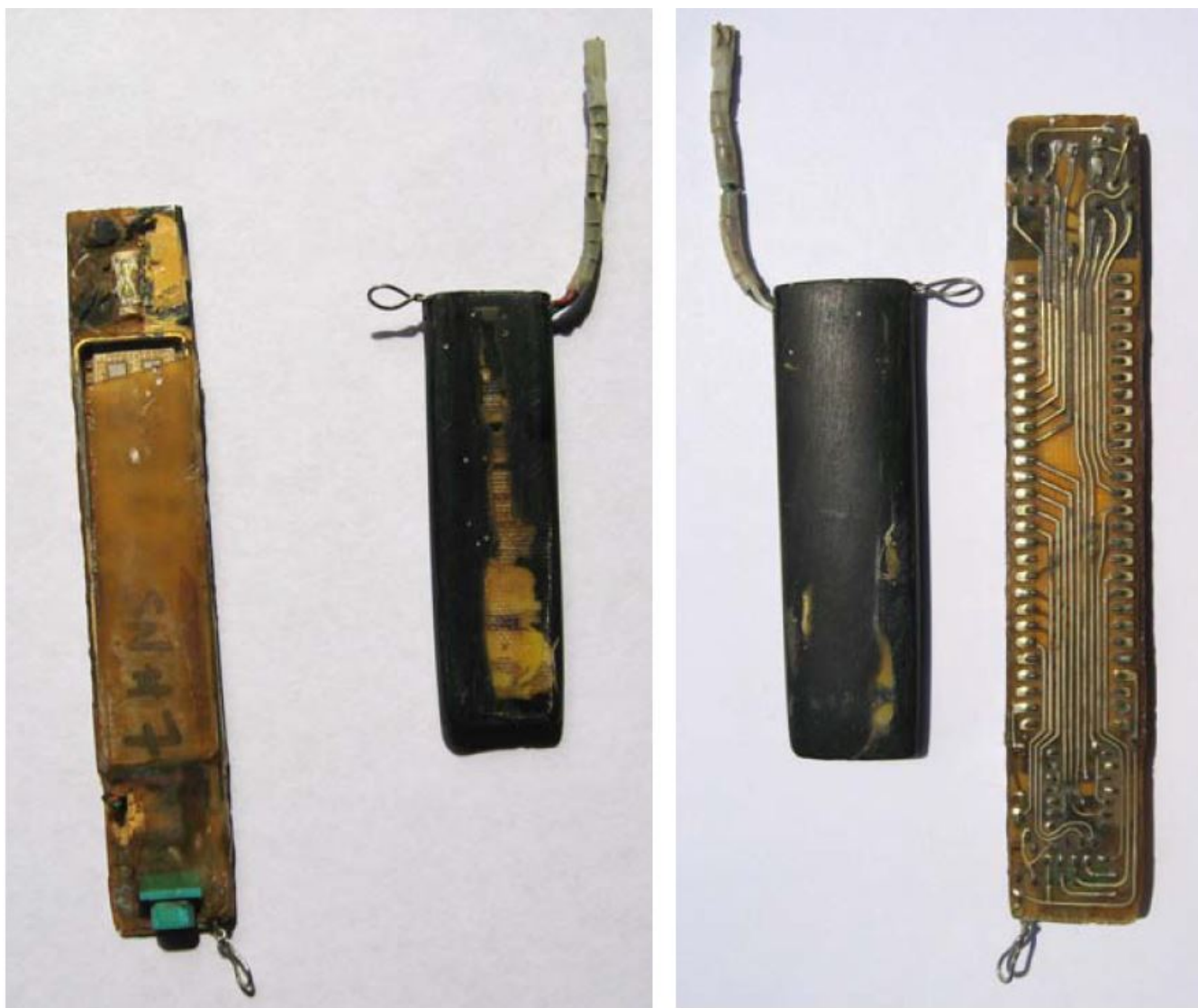
Figure 6-2. First Generation Temperature Tool. The logger electronics are on the outside and the battery pack is on the inside of each photograph..
