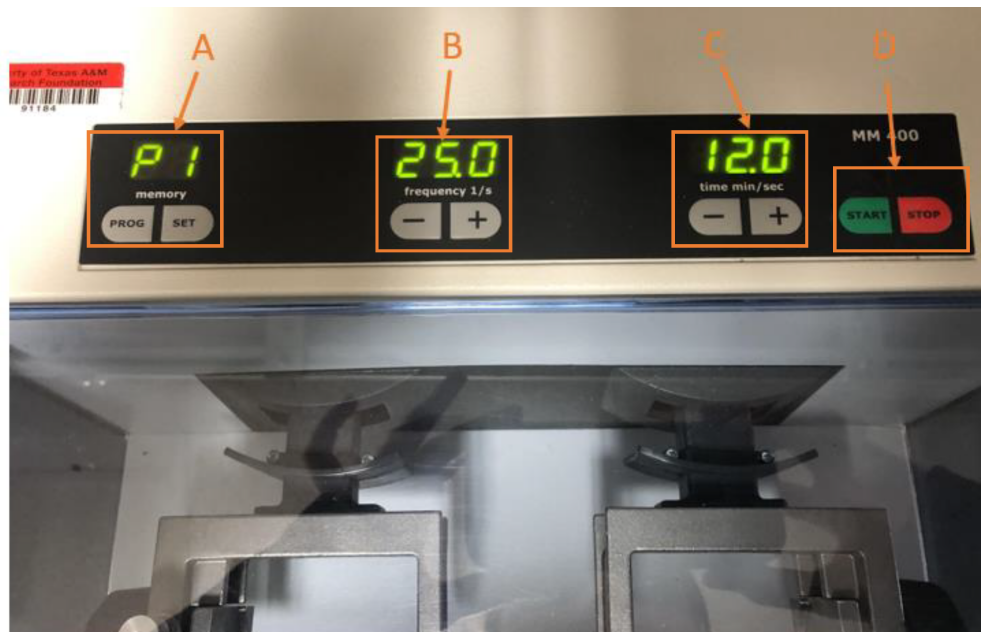
Figure 14. A. Preset programs. B. The shaker frequency. C. The time grinder is set for. D. The start and stop.
