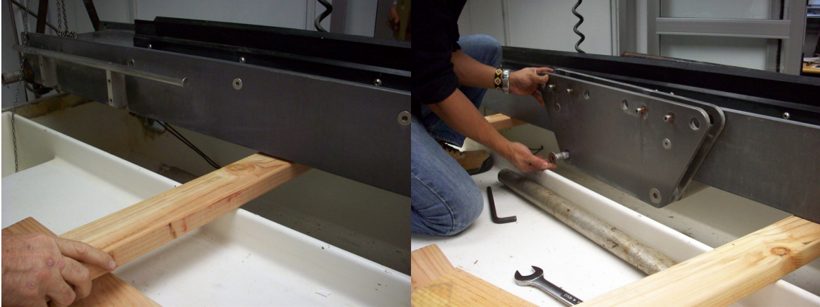
Left: Blocking of the starboard end of the splitter. Right: Removal of the side brackets of the splitting carriage.
