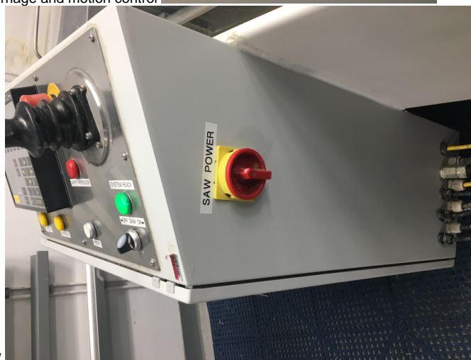
Main Power 110V. Turn on for power to carriage and motion control
