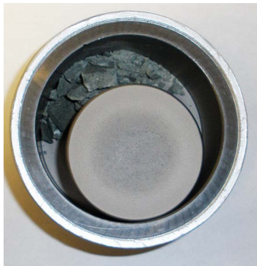
Figure 21. Small vessel filled with sample pieces. No sample material is on the top the puck or in the lid ring.
