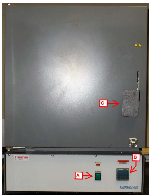
Figure 40. The Thermolyne Muffle Furnace. A. Power Switch B. Control Panel C. Door handle.
