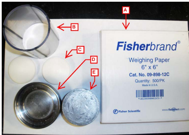
Figure 7: Materials needed for assembly of 'crushing unit'. A. Weigh Paper 6"x6". B. Core Liner C. Two Derlin Discs D. Stainless Steel Base E. Aluminum Die
