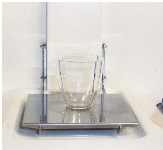
Figure 37. Weighing an empty inner crucible.
