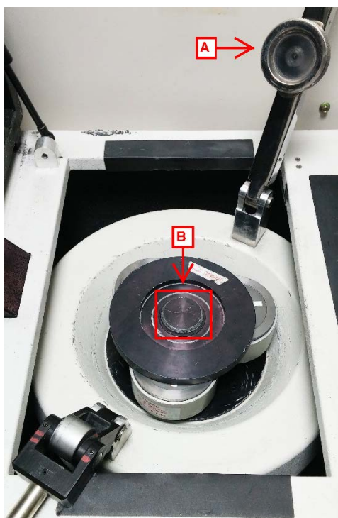
Figure 25. The top rack plate sitting on top of the three samples. A. Clamp arm. B. the “boss” of the rack plate, where the clamp arm will attach.
