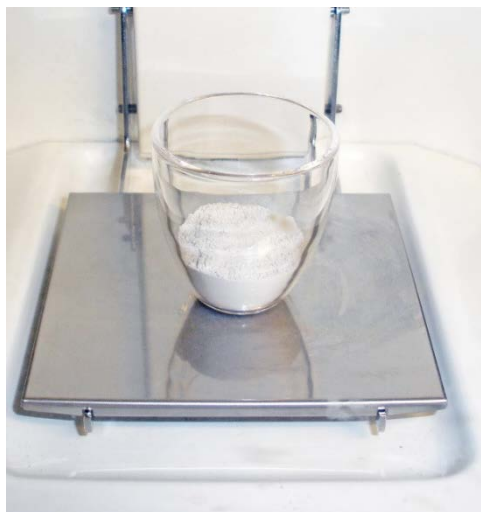
Figure 38. Crucible with approximately 5g of sample. Pre-ignition measurement
