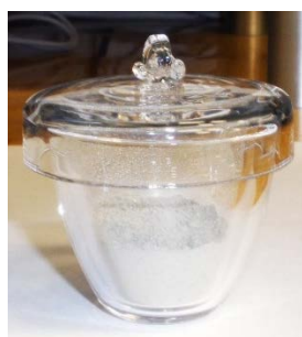
Figure 39. Complete crucible unit with sample, ready for ignition.
