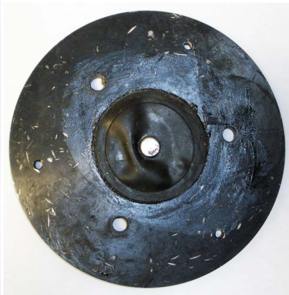
Figure 20. Single pinned rack plate to hold one small vessel in Shatterbox
