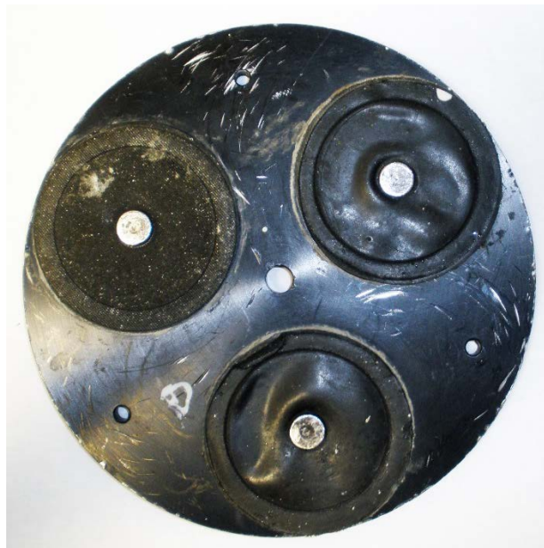
Figure 19. Three pinned rack plate to hold three small vessels in Shatterbox
