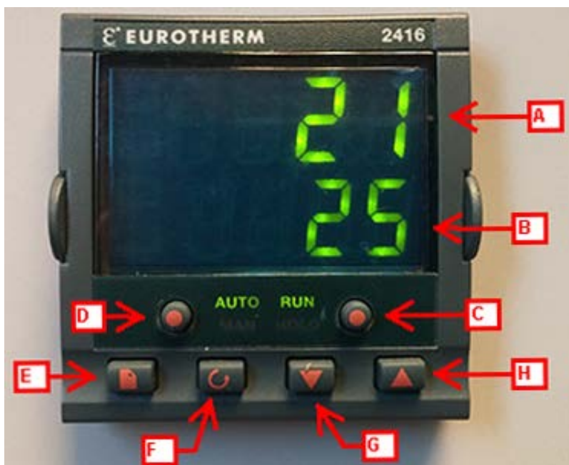
Figure 41. Control Panel on Thermolyne Muffle Furnace. A. Actual temperature. B. Desired/Set temperature. C. Run/stop button. D. Auto run button. E. Page button. F. Scroll button. G. Down button. H. Up button.
