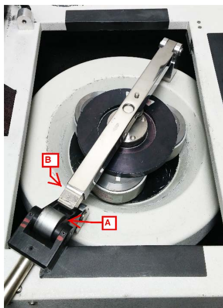
Figure 26. A. The lever arm inserted into the end of the clamp arm. B. The clamp arm pushed over the lever arm.
