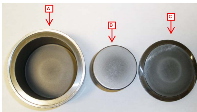
Figure 17. Small vessel components. A. Container B. Puck. C. Lid
