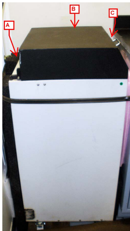
Figure 16. Shatterbox. A. Power switch. B. Cover. C. Control panel
