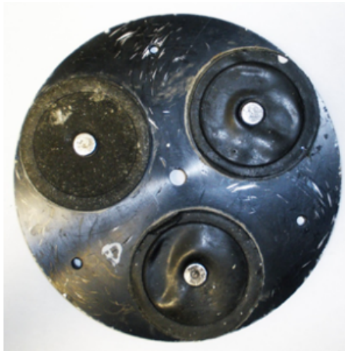
Figure 18. Three pinned rack plate to hold three small vessels in Shatterbox
