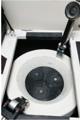
Figure 22. Inside the Shatterbox with the bottom three pinned rack plate resting inside the inner capsule.
