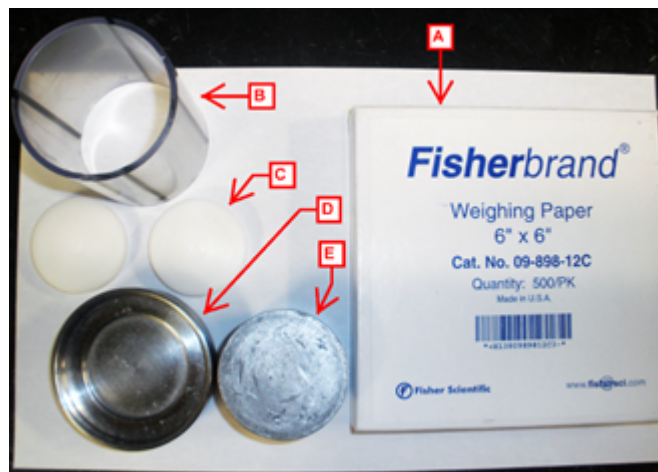
Figure 6: Materials needed for assembly of 'crushing unit'. A. Weigh Paper 6"x6". B. Core Liner C. Two Derlin Discs D. Stainless Steel Base E. Aluminum Die
