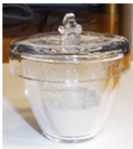
Figure 43. Complete crucible unit with sample, ready for ignition.
