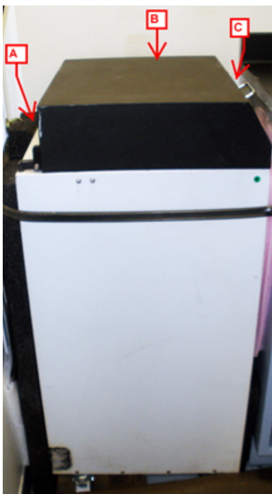
Figure 15. Shatterbox. A. Power switch. B. Cover. C. Control panel
