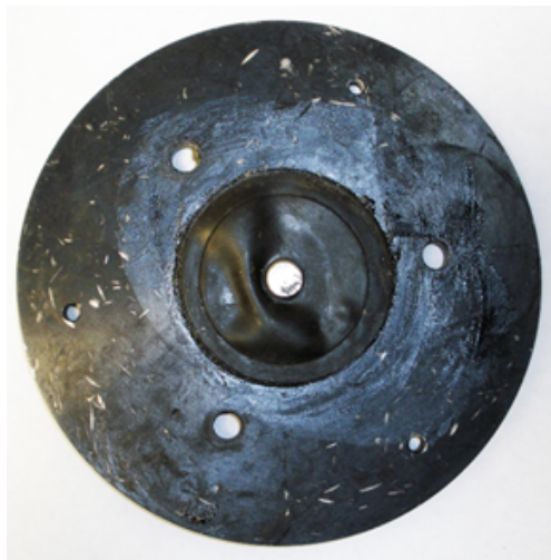
Figure 18. Three pinned rack plate to hold three small vessels in Shatterbox
