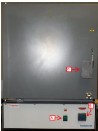
Figure 44. The Thermolyne Muffle Furnace. A. Power Switch B. Control Panel C. Door handle.
