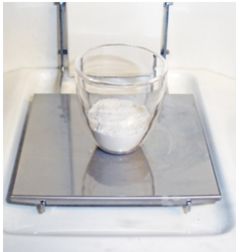
Figure 42. Crucible with approximately 5g of sample. Pre-ignition measurement
