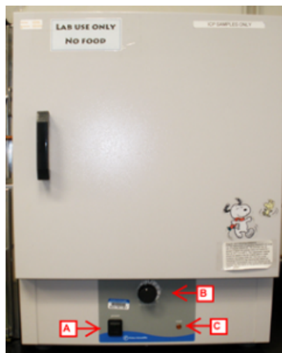
Figure 4. The ICP Prep Oven located in the X-Ray lab. A. 'On/Off' Switch B. Temperature Setting C. Heating Indicator
