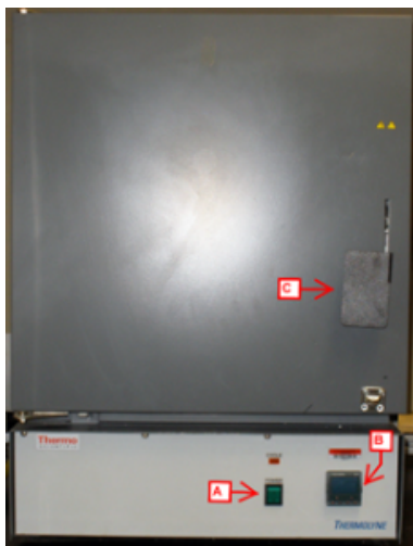
Figure 39. The Thermolyne Muffle Furnace. A: Power Switch. B: Control Panel. C: Door handle.
