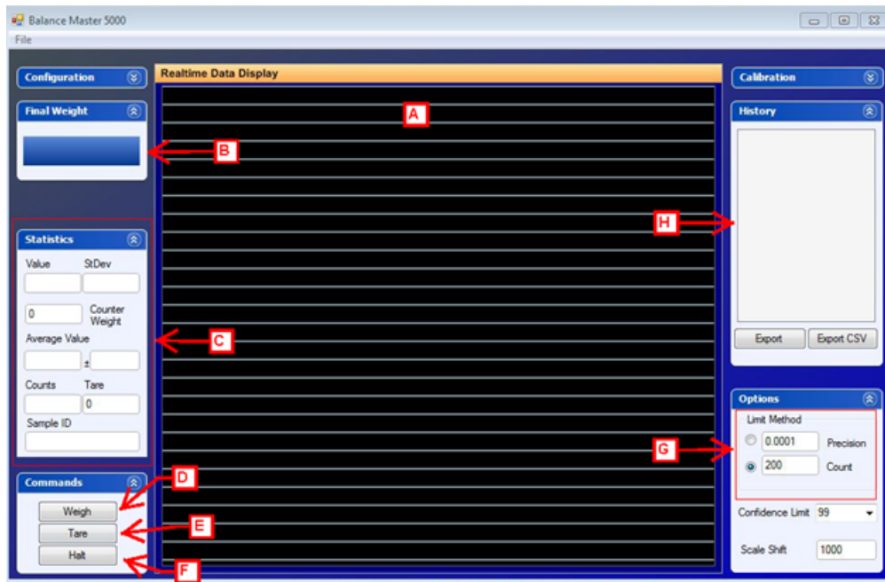
Figure 30. Mettler Balance program window. A: Graphical measurement window. B: Final weight panel. C: Statistics panel. D: Weigh. E: Tare. F: Halt. G: Options panel. H: History panel.
