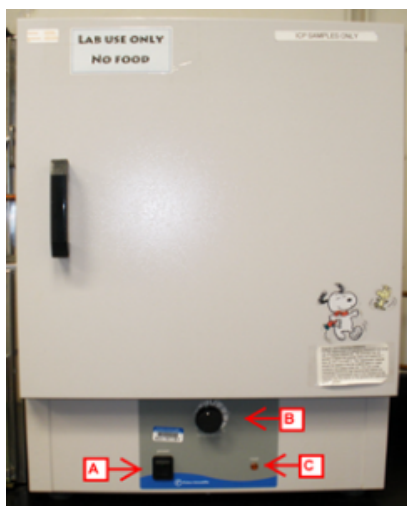
Figure 5. The ICP Prep Oven located in the X-Ray lab. A. 'On/Off' Switch B. Temperature Setting C. Heating Indicator.
