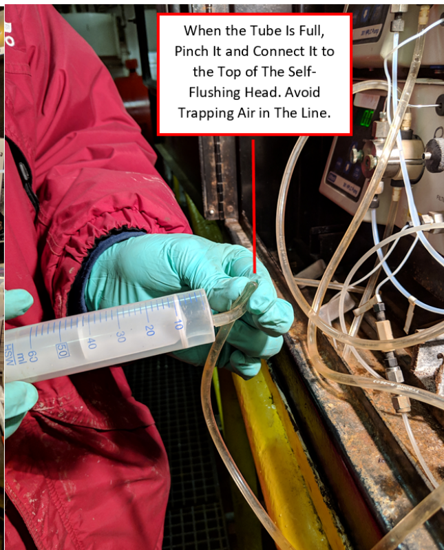
Priming & Flushing The Self-Flushing Head With Methanol
