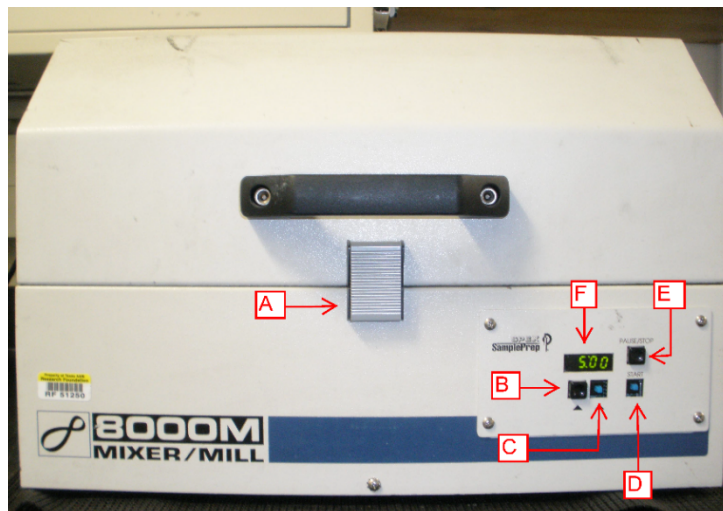
Figure 10: 8000 mixer mill. An older simplified version of the 8000M. Featured are the safety latch, timer dial, and start/stop button in the middle of the dial.
