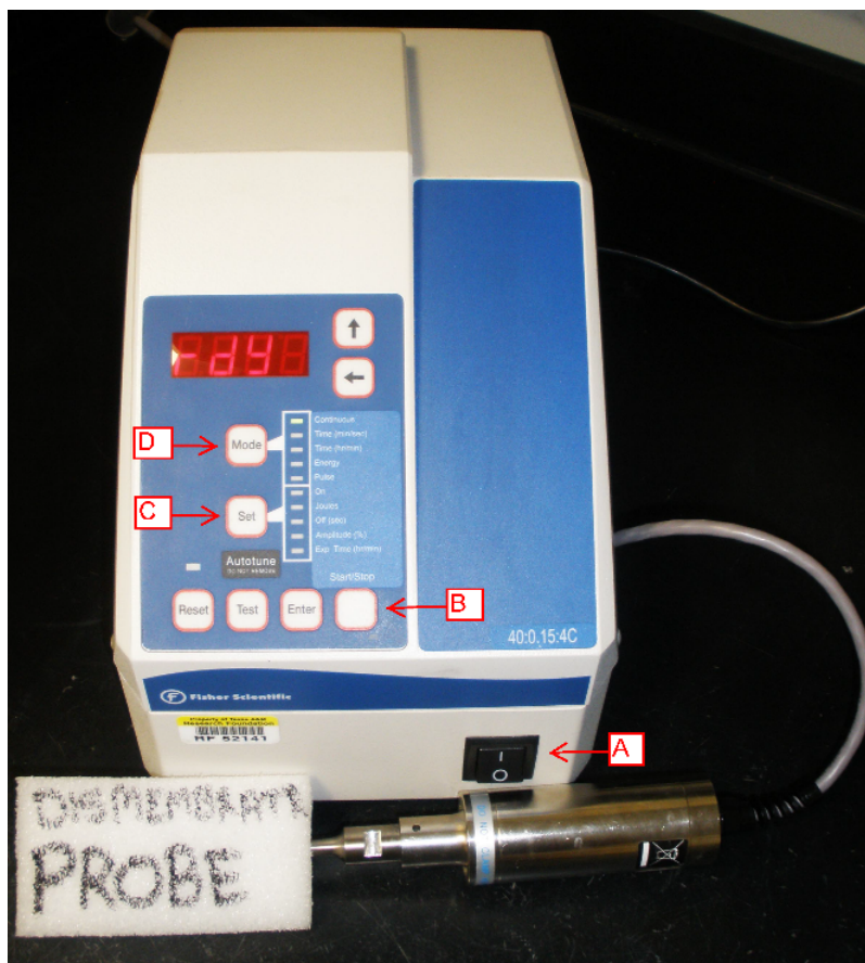
Figure 20: Dismembrator power source control Panel. (A) On/Off switch (B) Start button (C) Set button (D) Mode button
