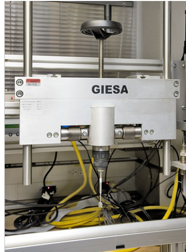
The Giesa FL2 Frame and blade component of the Automated Vane Shear (AVS) equipment.
