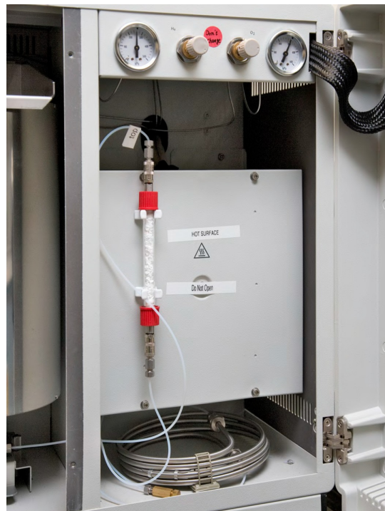
Figure 6. Detector Access: Protection Plate, GC Column (inside), Adsorption Filter WARNING: The GC column may only be serviced by the shipboard technicians
