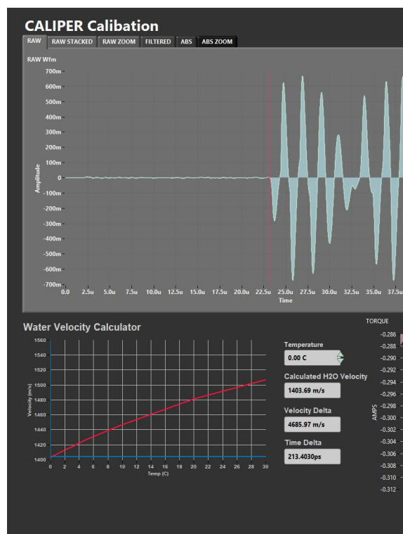
Figure 10. Caliper Calibration Windows. Raw data graph tab (left) and the ABS zoom graph tab (right)
