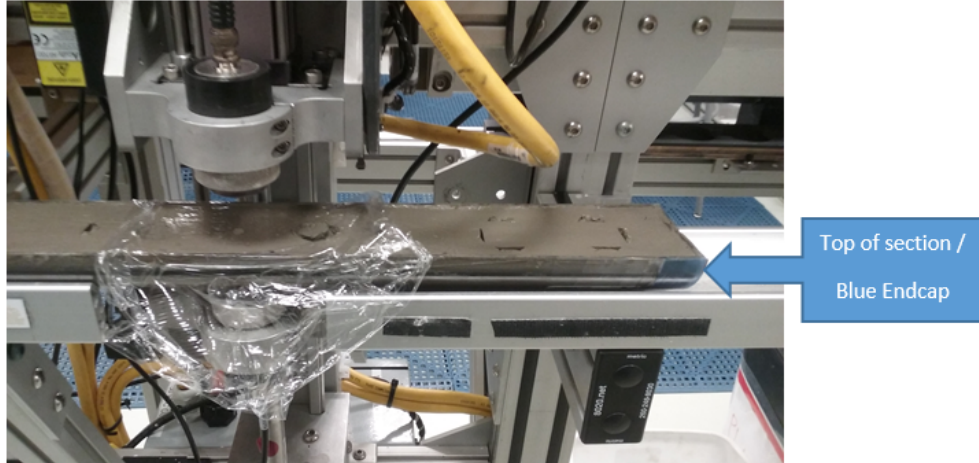
Figure 4. Section-Half loaded under caliper.
