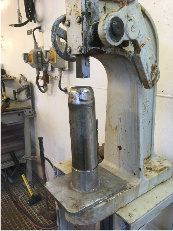
Figure 5: Metal disc for pushing on core material
