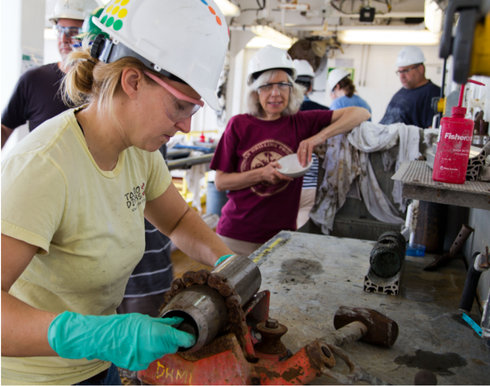
Figure 1: Extruding core catcher material at the core catcher bench; notice the Paleontologist waiting with white bowl – give PAL sample to paleontologist.
