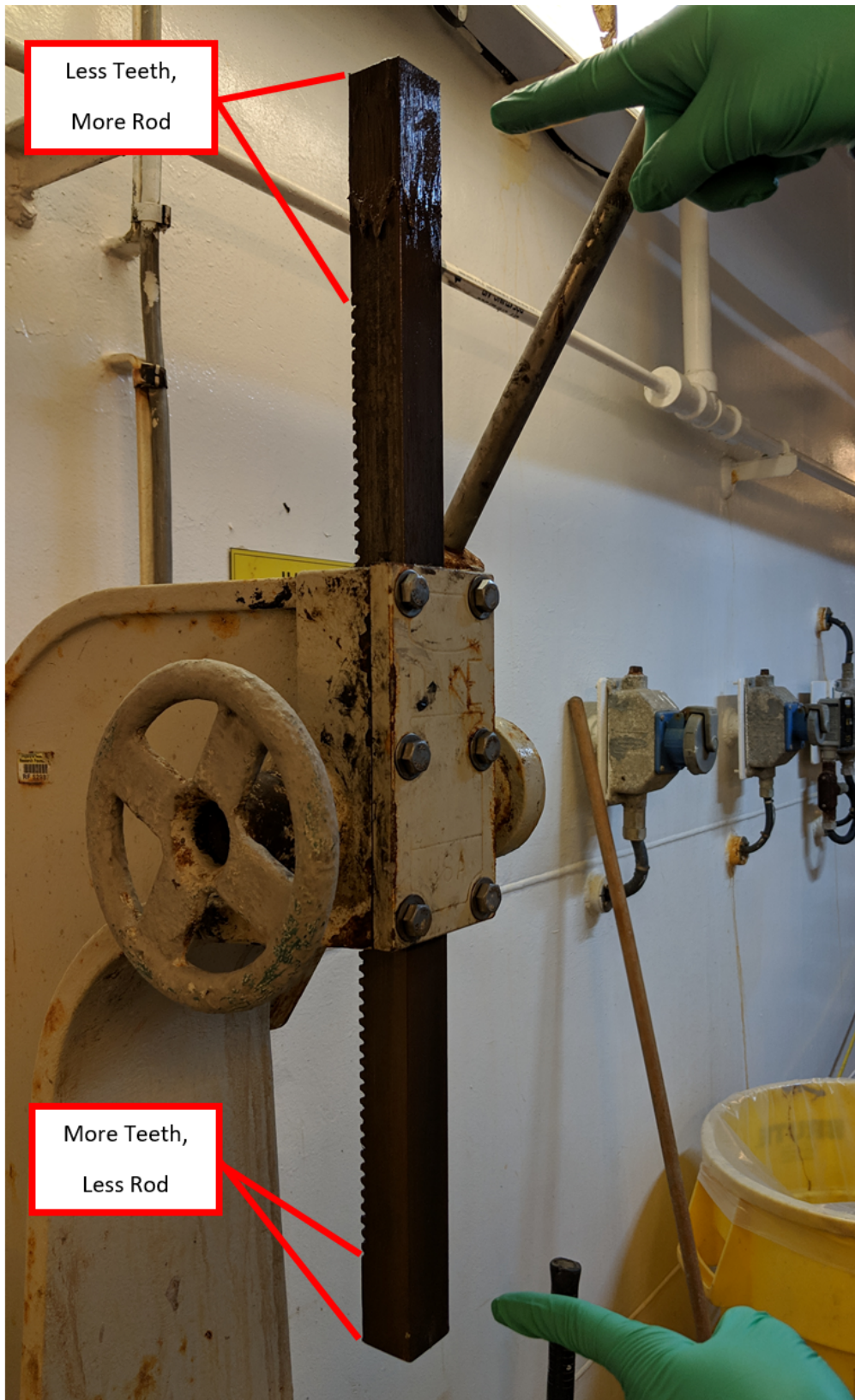
Figure 7: Toothed Square Rod, Proper Configuration
