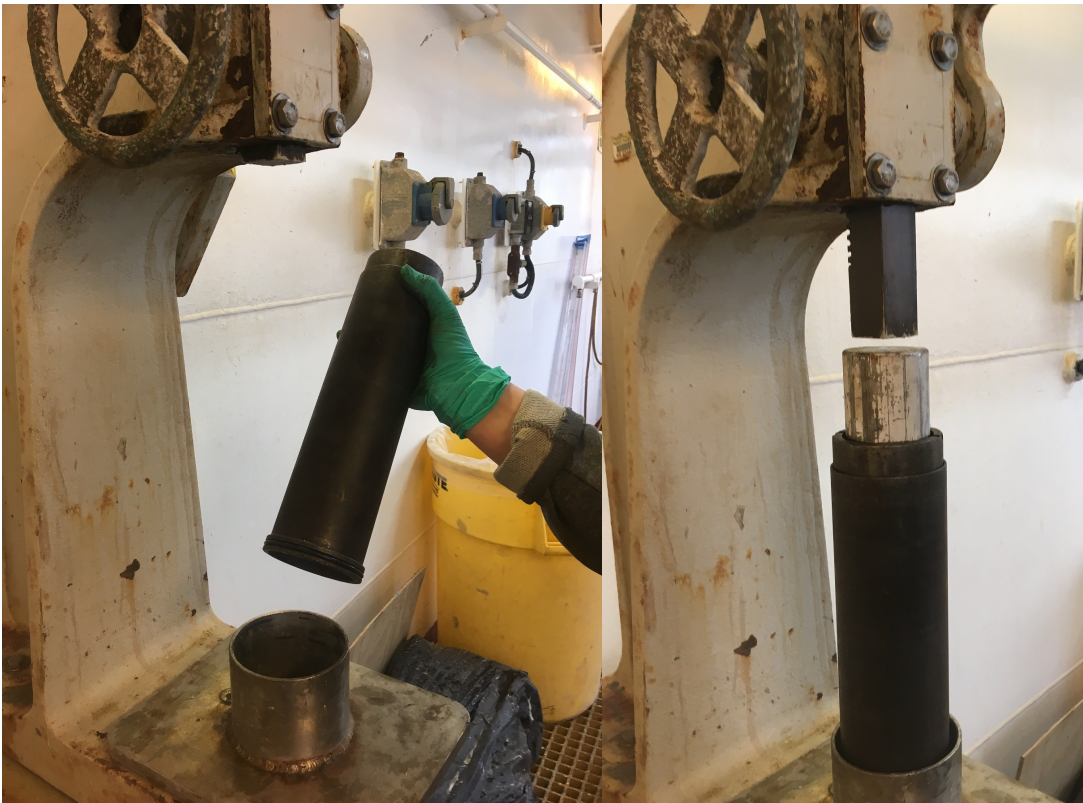
If the press is unavailable the old XCB sleeve tool needs to be used to get the inner rings out of the sleeve. Note that the sleeve must be turned around on the chain vice to get the lip of the flange to catch the vice and be stable.
