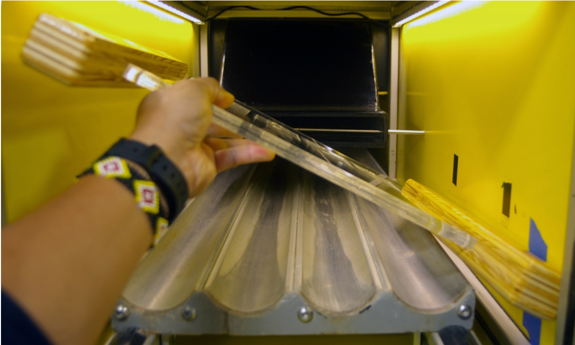
Photo 5: Tilt the tray sideways and pull it out through the diagonal of the chamber.
