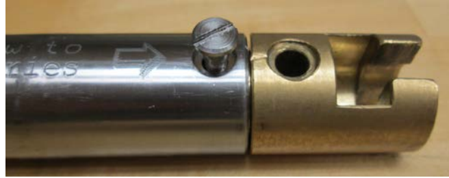
Fig. 2.1b. Replace end cap and secure with shoulder screw
