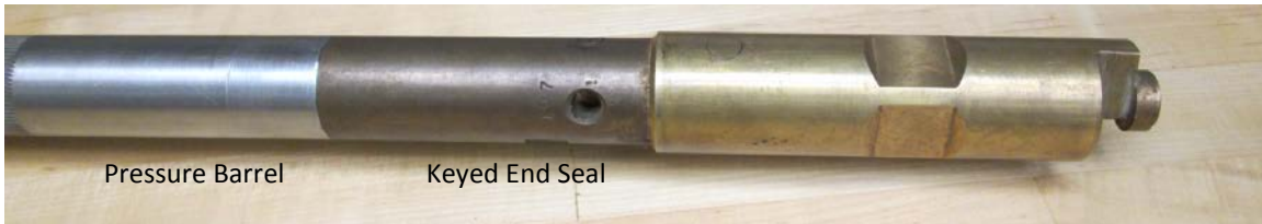
Fig. 3.3- End seal in place at end of pressure barrel
