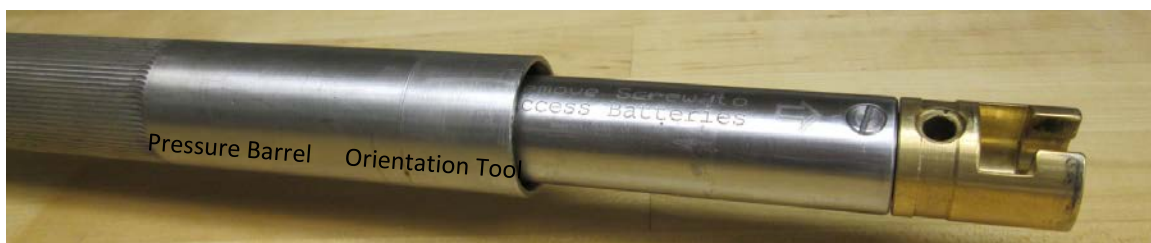
Figure 3.1- Orientation tool in Pressure Barrel
