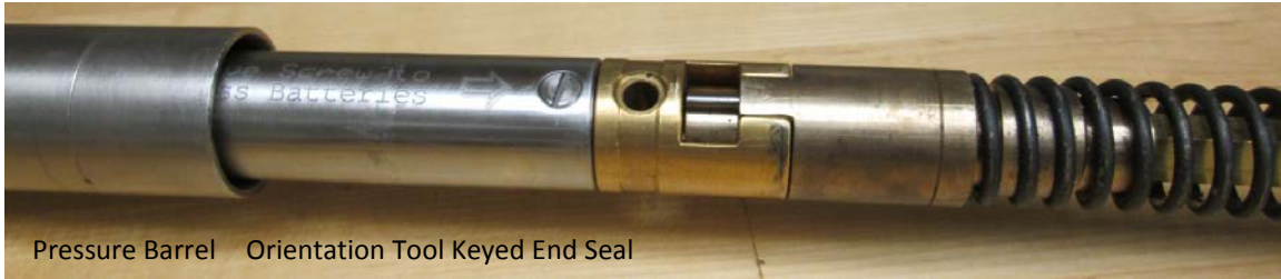
Fig. 3.2- Keyed End Seal connected with Orientation tool
