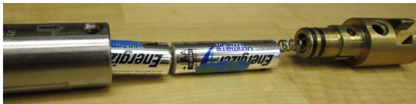
Figure 2.1a. Insert batteries positive end first
