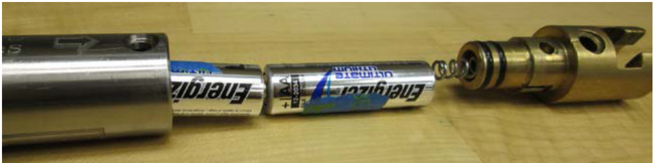
Figure 2.1a. Insert batteries positive end first
