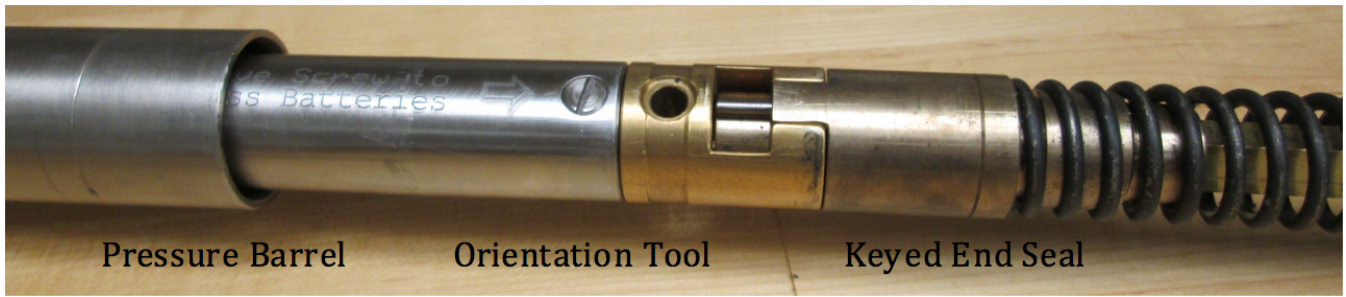
Fig. 3.2- Keyed End Seal connected with Orientation tool
