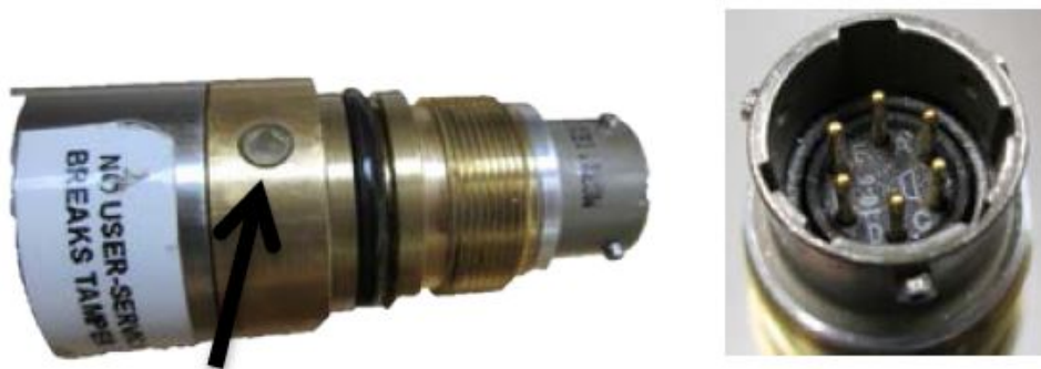
Figure 1.2a. Communications port end (without cap); arrow indicates LED
