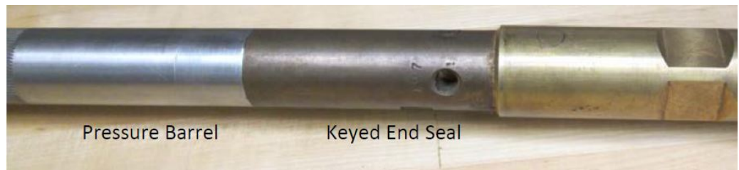
Fig. 3.3- End seal in place at end of pressure barrel
