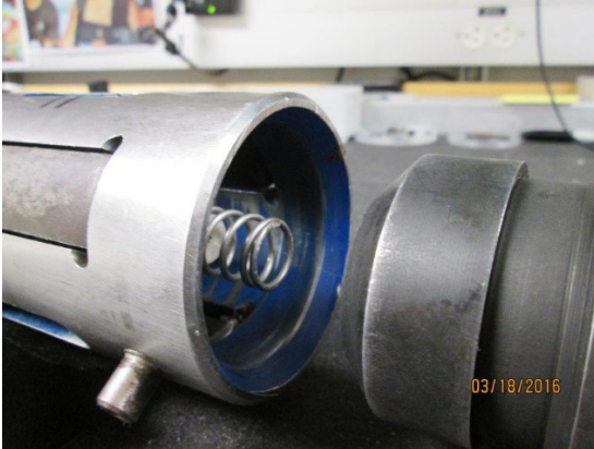
RS-latch with plug, pulling neck
