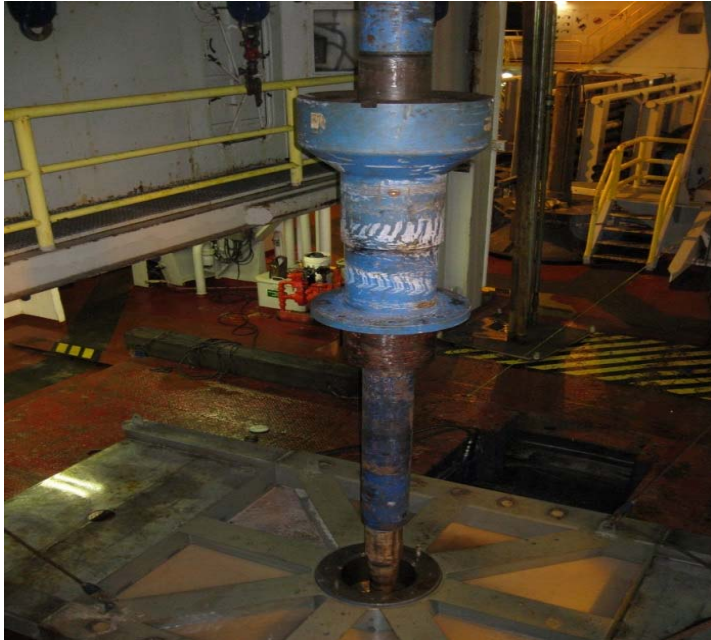
The HRT top assembly; the Base Adapter and casing are landed in the Mud Skirt.
