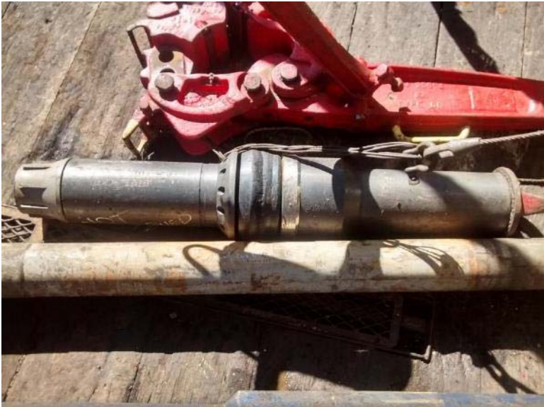
Top; The 10-3/4 Cup Packer. Btm; The cup showing erosive wear after one of the casing runs.
