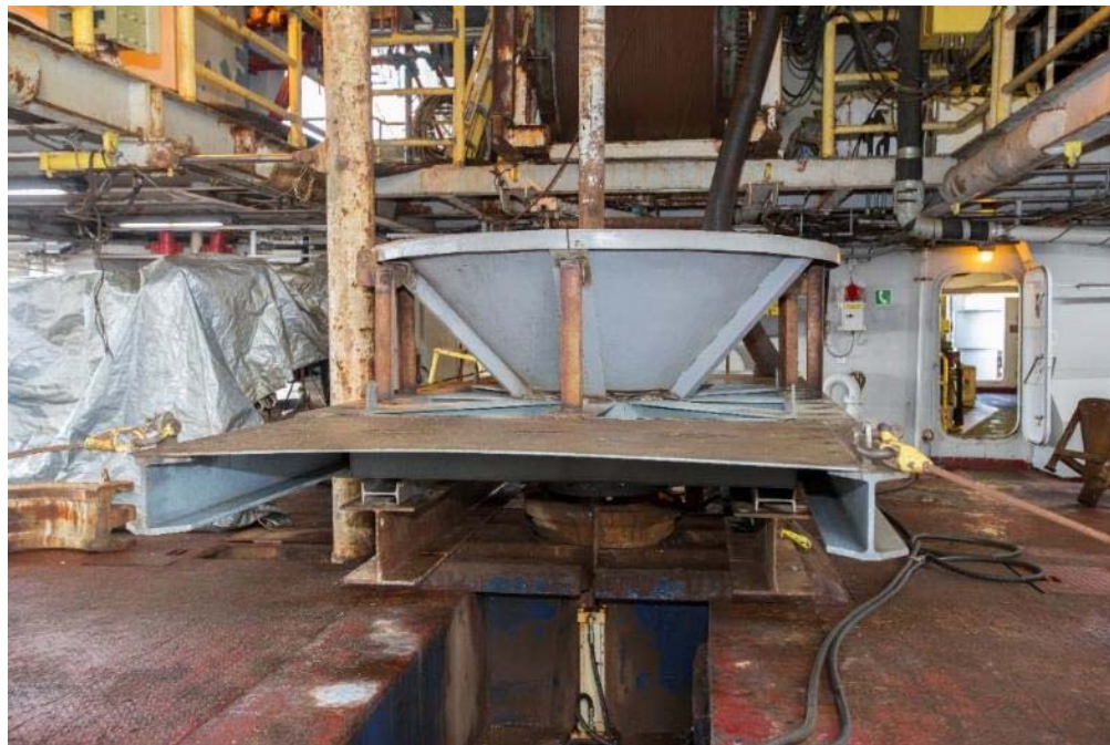
The base with funnel. Note the height of the funnel has been “chopped” down. Also, additional struts have been added.
