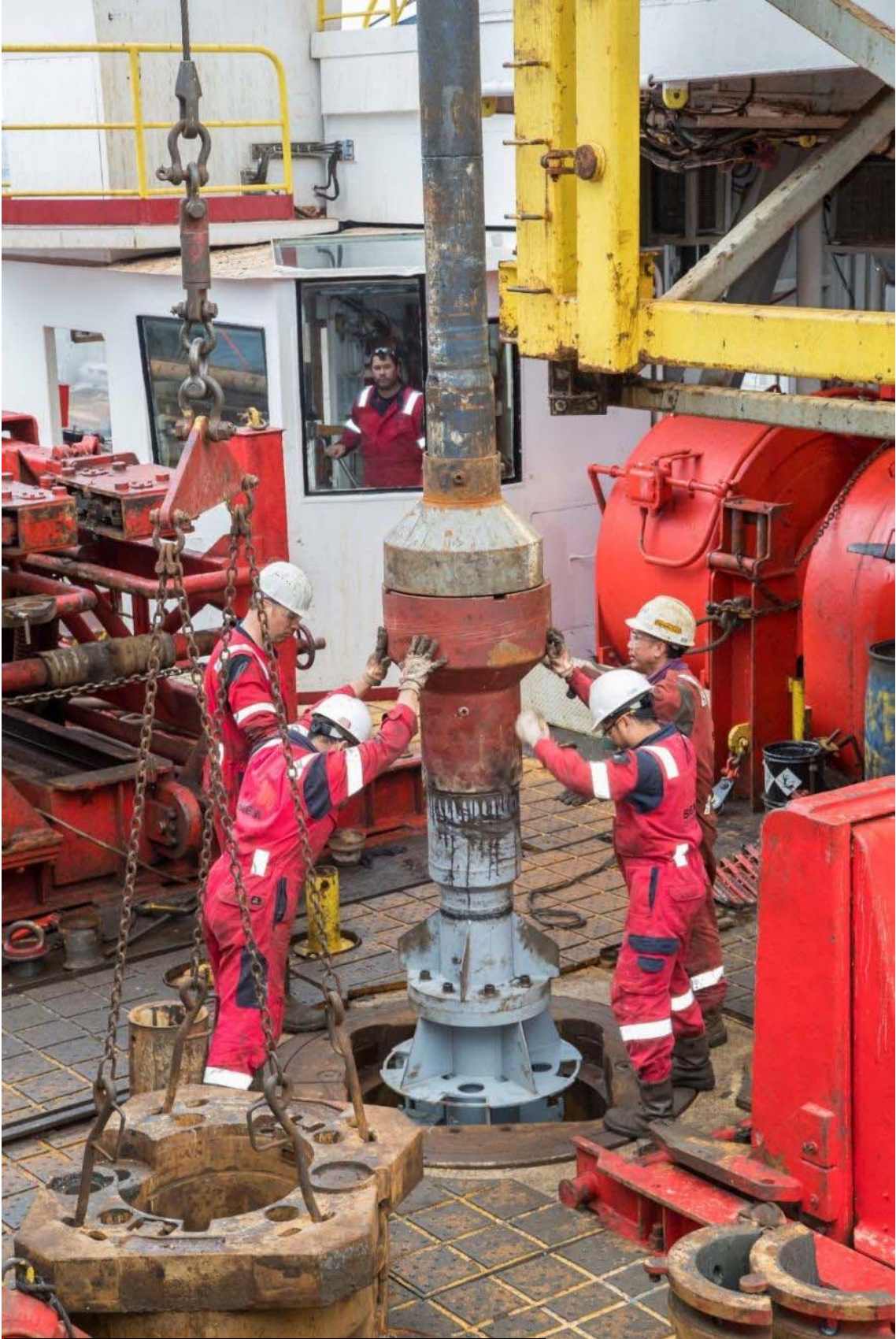
The ACORK being lowered through the rig floor.
