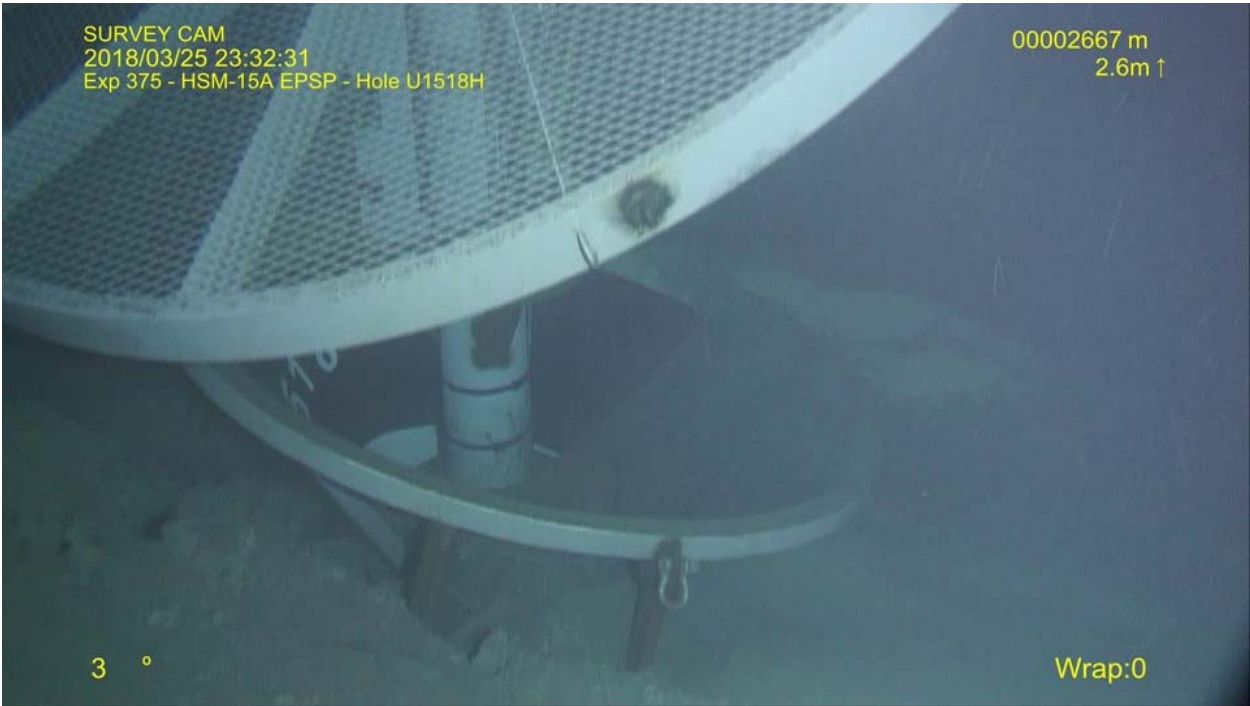
The ROV Platform hung above the valve bay on U1518H.
