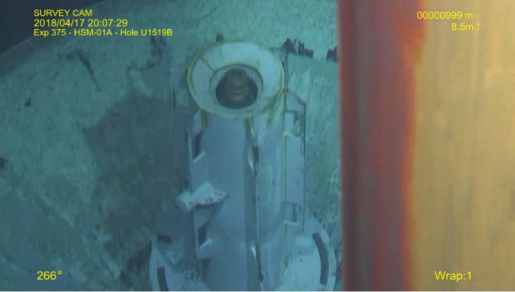
U1519B, from the top; The damage to the CORK-II, the valve bay, and the top plug landed.
