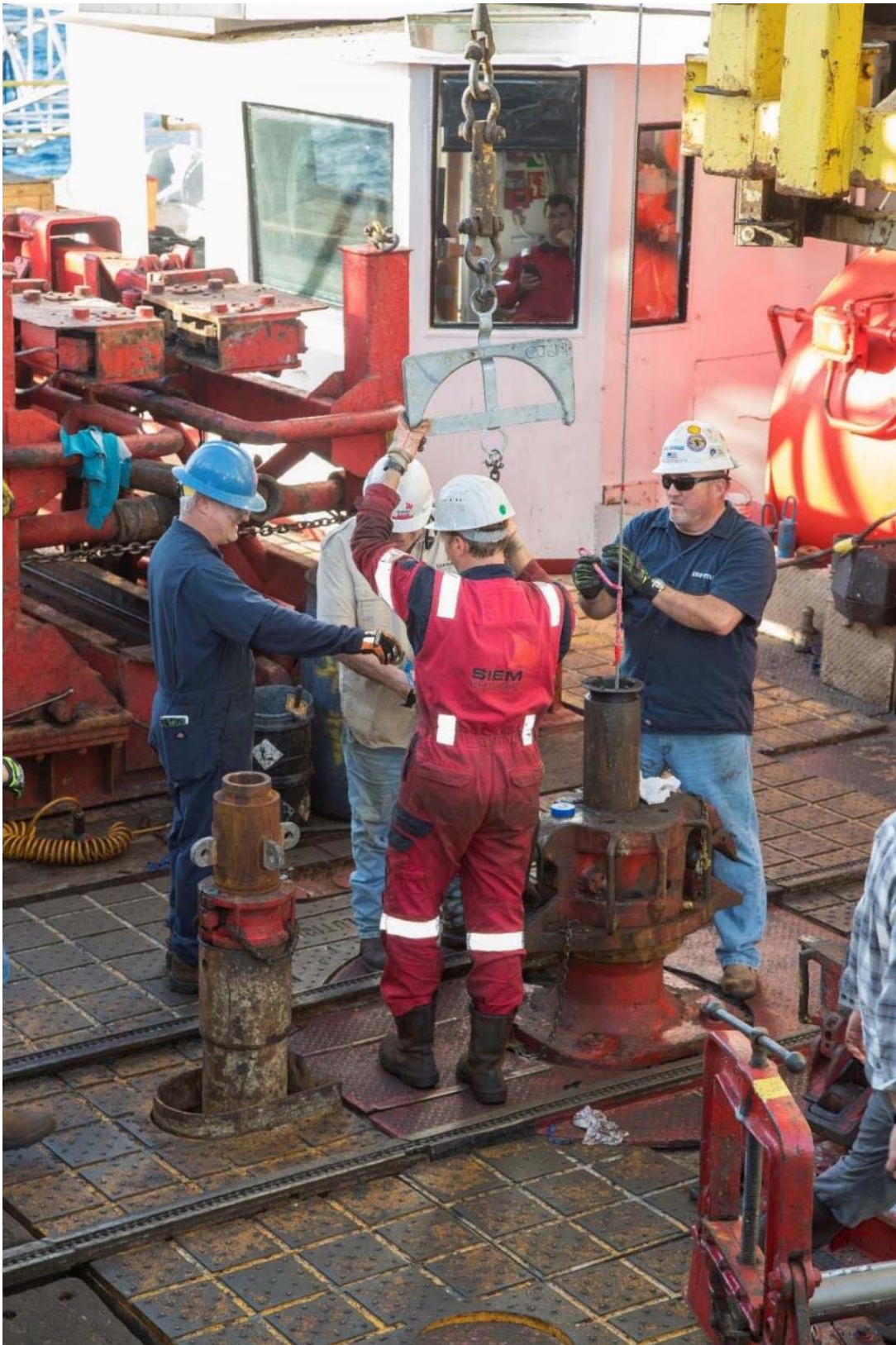
The instrument string being deployed on U1518H, using the lifting bales.
