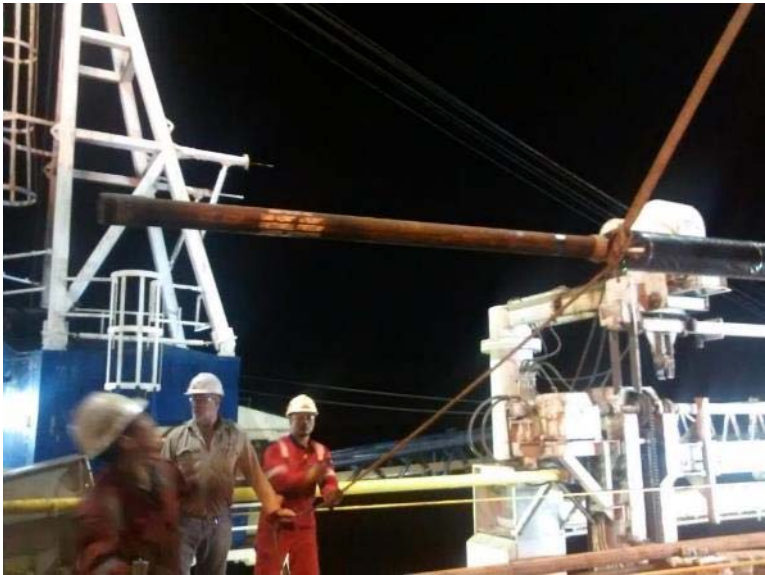
The U1518H swellable packers being swung forward from the helipad and the protective wrapping removed at the rig floor.
