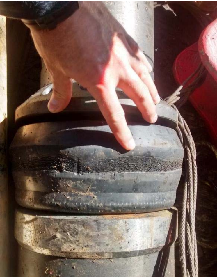
Top; The 10-3/4 Cup Packer. Btm; The cup showing erosive wear after one of the casing runs.
