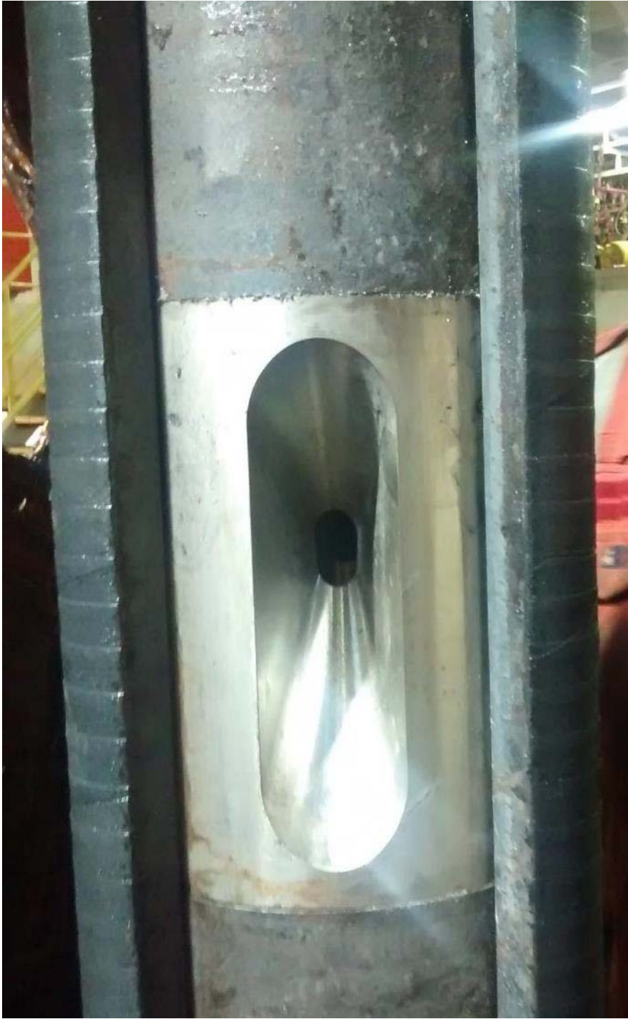
The quadrant seal. Note the proper orientation of the osmo seat.
