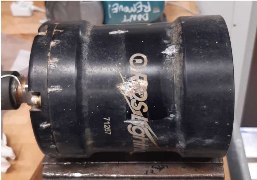
Pitting on ROS LED Light
