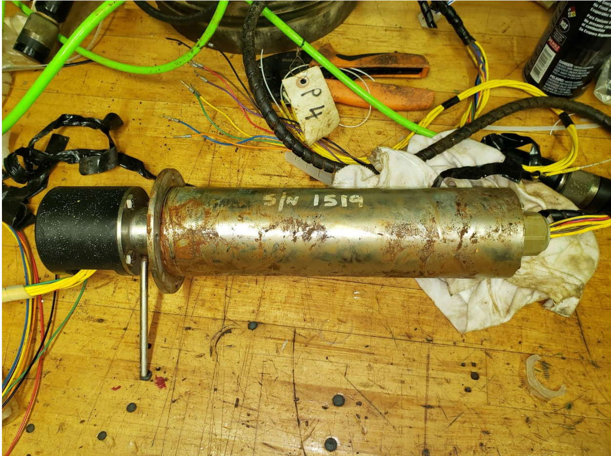
Figure 19. Alpha Slip Ring Serial Number 1519 taken out of service and returned for repair.
