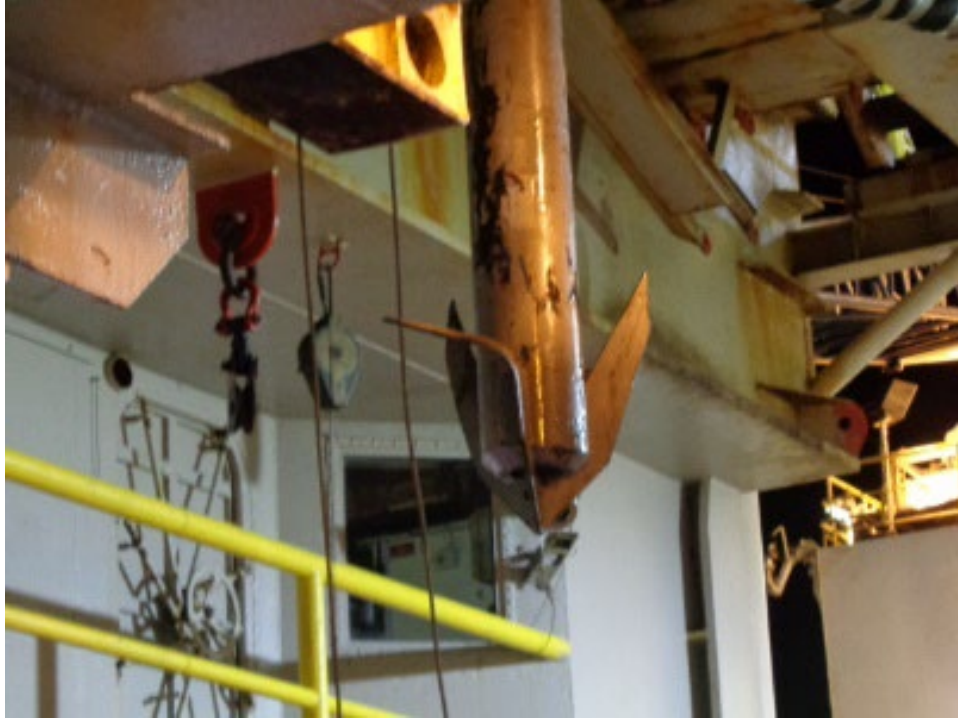
Figure 18 Bent Hook and No 504B Platform
