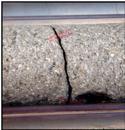
Figure 4 - Hard rock core with hatch marks.
