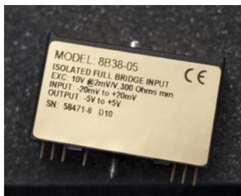
Figure 8. Isolated signal conditioning module.
