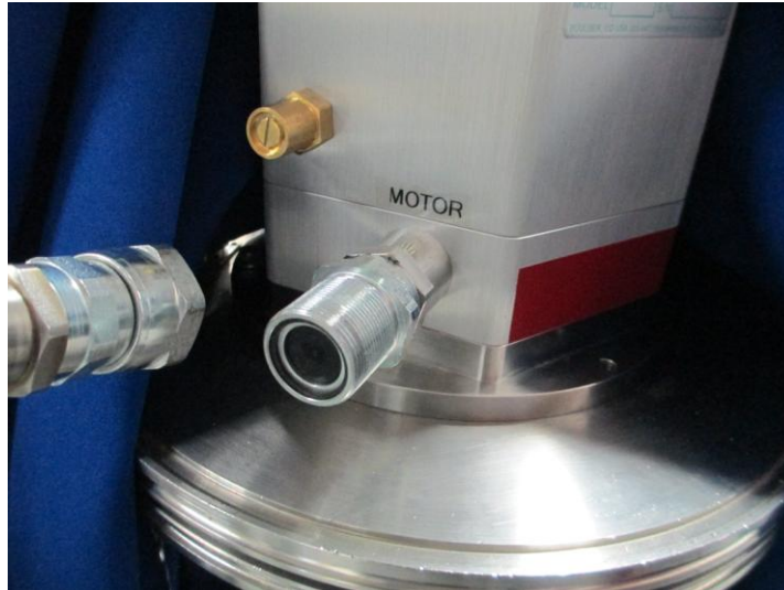
Figure 6-3: Connecting the remote motor assembly's flex line to the PT 403/5/7 cold head
