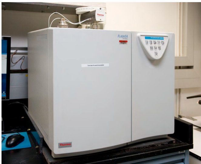
Figure 2. Top and Front Instrument Panels. (Dry Sample Autosampler is located on top of furnace.)
