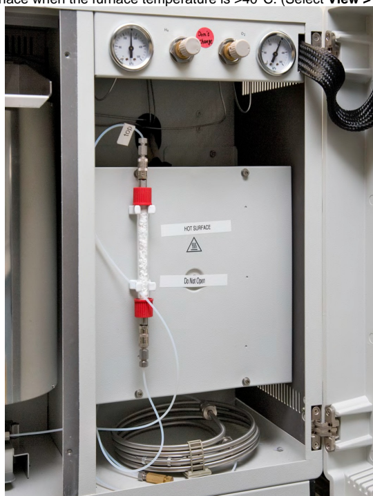
Figure 6. Detector Access: Protection Plate, GC Column (inside), Adsorption Filter.
