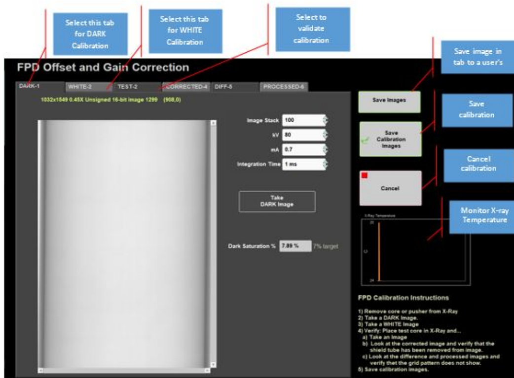
Figure 21- Detector Calibration user interface window. From this utility a user may take necessary calibration images and test the corrections prior to applying them to images.
