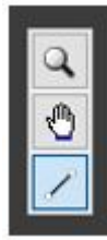
Figure 32- ROI tool available in the image processing utility. The histogram or line profile will be displayed when the ROI tool is used. A line will produce a line profile. A box will produce a histogram.
