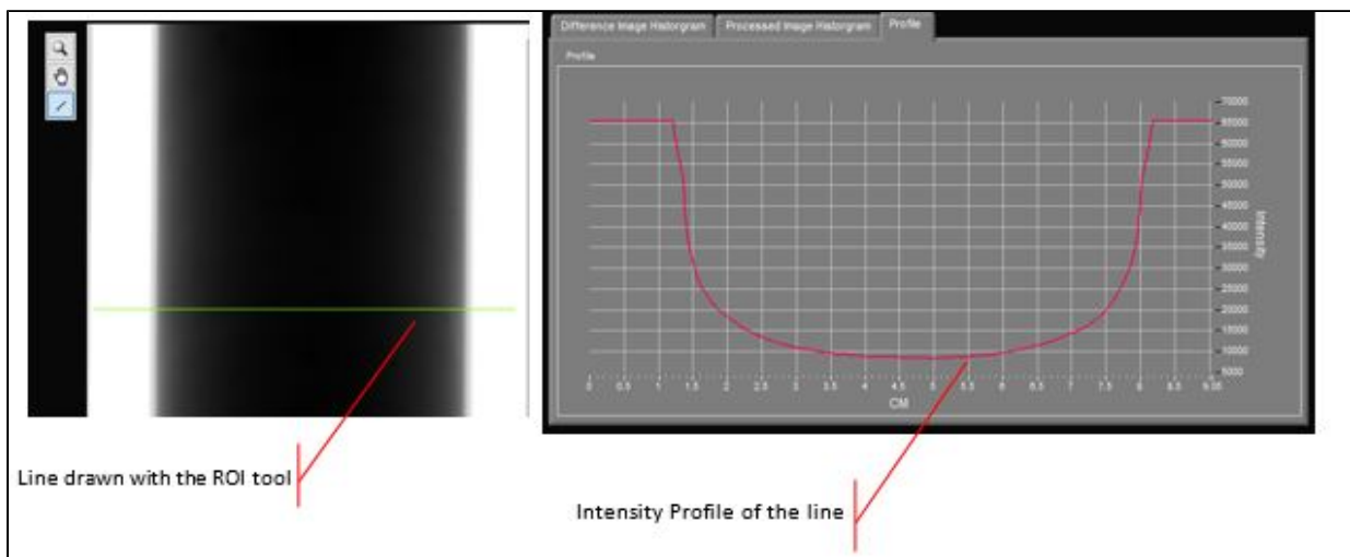
Figure 33- Example of ROI tool used on a raw image and the resulting intensity profile.
